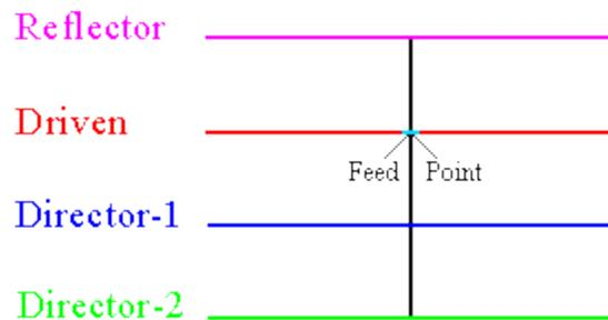
The driven element is cut into two halves and insulated from the boom with non-metallic material. Then the two wires of the coax are connected, one to each section of the driven element. You may drill small holes and use sheet metal screws to accomplish this.
