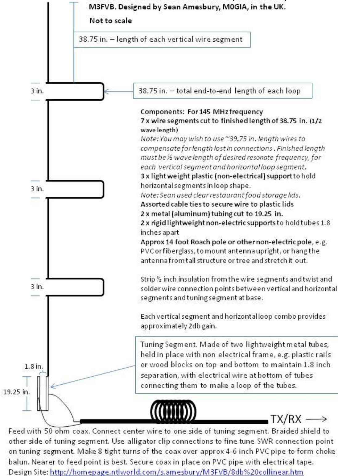
A more detailed build instruction set for this 8 db portable co-linear antenna is at:
